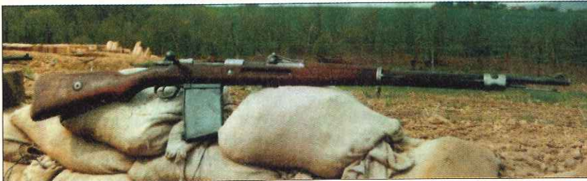
Some specialty arms were developed for the trenches. This rare Gew98 Mauser has an extended 20-round magazine, giving the soldier 15 extra shots before reloading.
