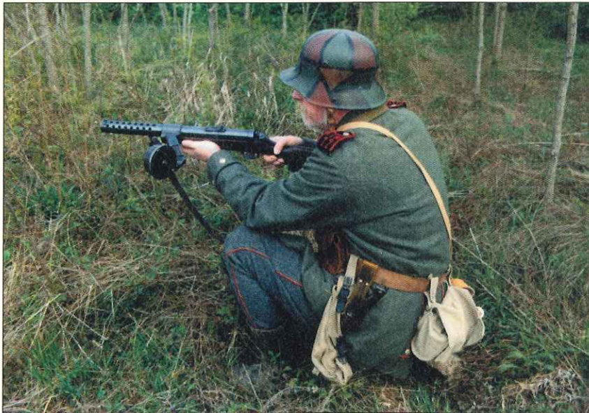
Though some were on the drawing boards and under development, despite being ideal for trench raids, few sub-guns were used during World War I. The one seen the most was the 9mm German MP-18 Bergmann. Its "snail-drum" magazine held 32 rounds.
